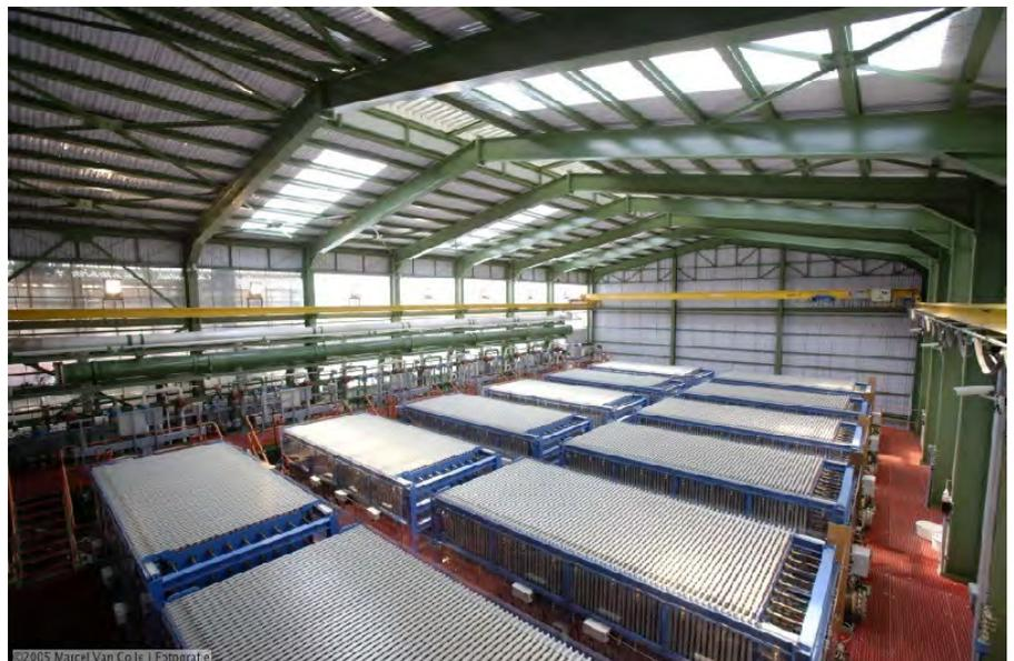
Membrane electrolysis for chlor-alkali production, without use of mercury, courtesy of Solvay
