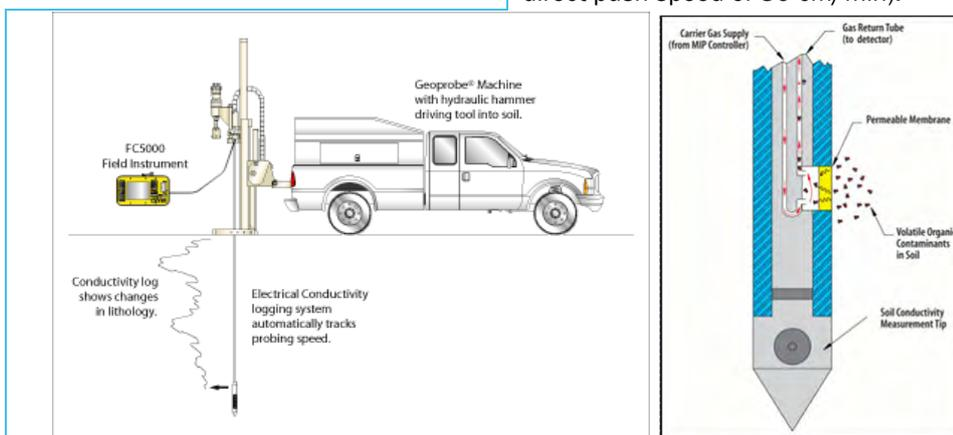
EnISSA concept: direct push; local heating of soil; hydrophobic semi permeable membrane; inert carrier gas; and transport to detector
