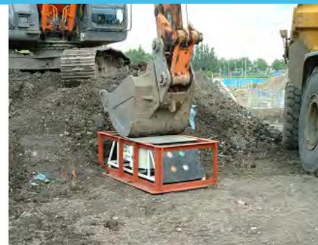
**The GEM system in operation with the loaded excavator bucket placed over the detector**
