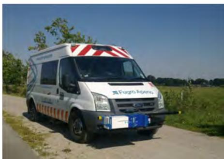
Medusa: spectral gamma sensor mounted on the front of the measurement vehicle. The EM sensor is mounted behind the vehicle in a non-conductive carriage. The GPR is mounted under the vehicle.
